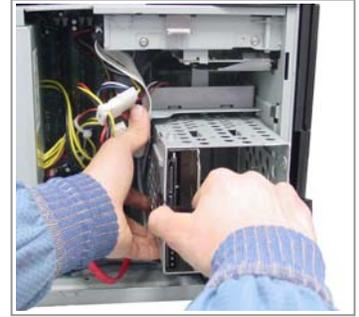
**Step 5.** Release the HDD bracket enclosure by pulling the black handle as shown. Some force may be required to unlock the handle. Slide the complete HDD bracket enclosure out of the unit.
