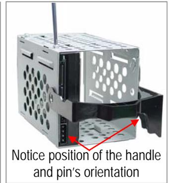
**Step 6.** Using the enclosed magnetic screwdriver, remove the four (4) screws that secure the hard drive into the bracket enclosure. **IMPORTANT! Before proceeding, take note of original position of the drive inside the bracket.** Slide out the original drive.
