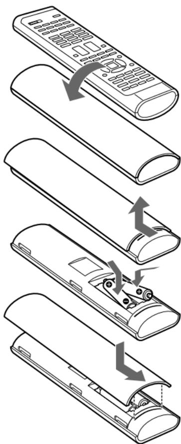
Insert the batteries (negative end first) through the guide clamp within each compartment as shown above.
