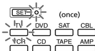
While the Hold function is on, no function can be operated. (The SET button and the Component Select button currently selected flash twice.)
