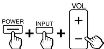
When pressing the POWER button and the INPUT button, all the Component Select buttons go off. When pressing the VOL - button while holding down the POWER button and the INPUT button, the SET indicator lights up and the Component Select buttons light up one by one. When the SET indicator turns off at last, all settings are cleared, and the Commander returns to its original state.
