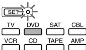
When you “teach” signals to the SYSTEM CONTROL buttons, you can release the SYSTEM CONTROL button when the SET indicator lights up. The SET indicator lights up, but the SYSTEM CONTROL button does not light up.
