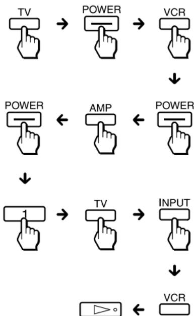
You can program up to 16 consecutive steps on each of the Component Select buttons, including the first step of pressing to select a Component Select button.
