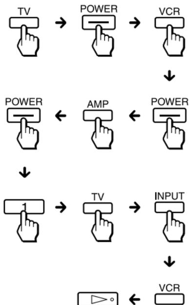
You can program up to 16 consecutive steps on each of the SYSTEM CONTROL buttons (1 – 4), including the initial step of pressing switch to a Component Select button.
